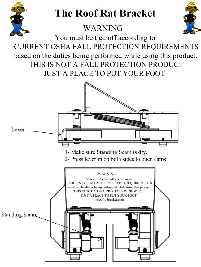
3- With cams open, set bracket firmly on deck with standing seam in between the cams, release lever.
